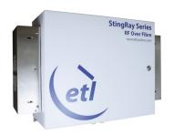
The StingRay RF over Fibre Outdoor unit (ODU) is a robust weatherproof (IP65 rated) enclosure which has been designed to be wall or post mounted close to the antenna. It can accommodate up to 10 Transmit or Receive 200 series StingRay Fibre modules.
